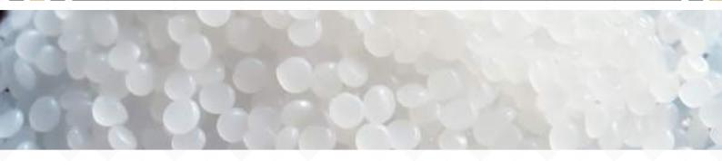
Characteristics: Linear Low Density Polyethylene (LLDPE) is known for its linear structure with short chain branches, providing excellent puncture and tear resistance. This polymer combines the flexibility of Low Density Polyethylene (LDPE) with the strength and durability of High Density Polyethylene (HDPE).
