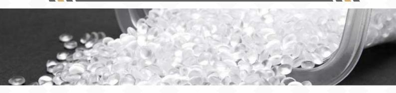
**Characteristics:** High Density Polyethylene (HDPE) is recognized for its high strength, stiffness, and excellent chemical resistance. HDPE's tightly packed crystalline structure gives it superior mechanical properties, making it suitable for heavy-duty applications.
