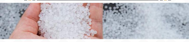
**Characteristics:** PET is a transparent, lightweight, and FDA-approved plastic widely used in food and beverage packaging. It boasts high impact strength and a good gas and moisture barrier, ensuring product freshness.
